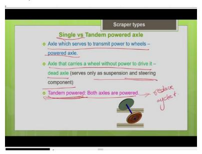
So, now let us see what are these are single versus tandem powered axle scrapers? So, axle basically how do you classify the axle into powered axle and dead axle? See in our common vehicle say for example car, so you know that it may not be the case like all the axles are powered. So, maybe we only one axle may be powered the other axle we just dead ok powered in the sense the powered axle will transfer the power to the wheel those wheels are called driving wheels.
